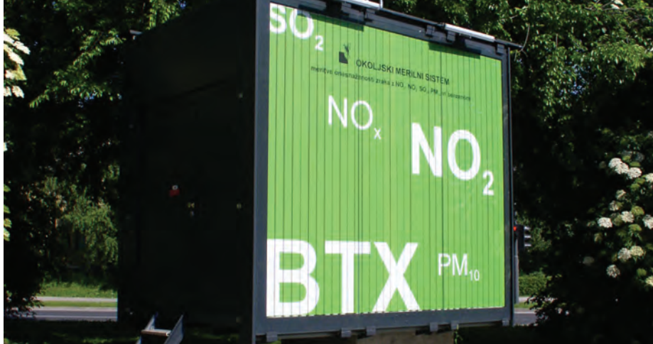
Monitoring station in the centre of the city intended for monitoring traffic pollution.
