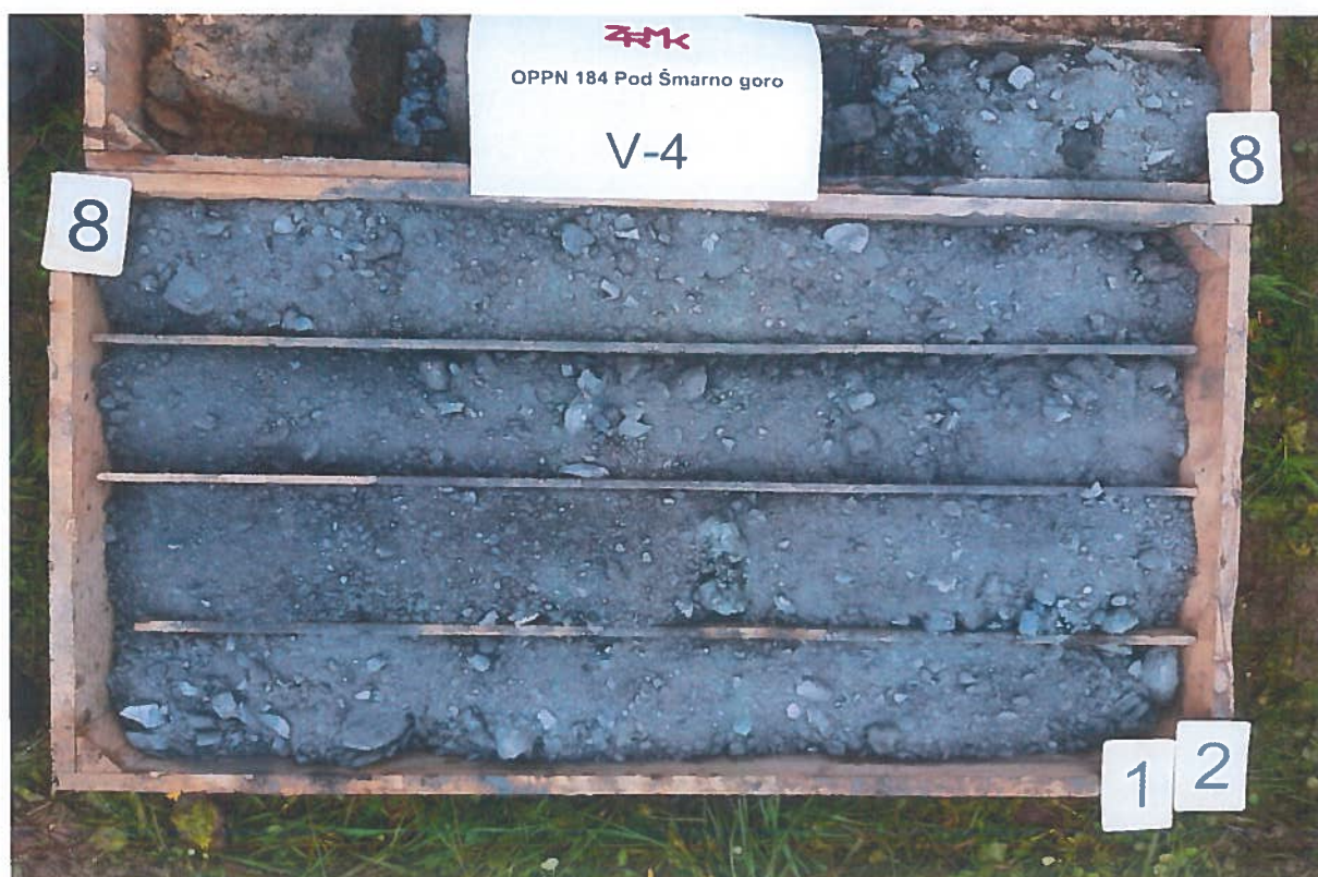
Slika 7: Sondažna vrtina V-4 (8,0 m – 12,0 m)
