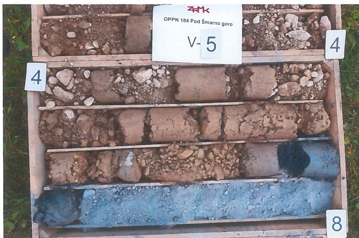
Slika 9: Sondažna vrtina V-5 (4,0 m – 8,0 m)
