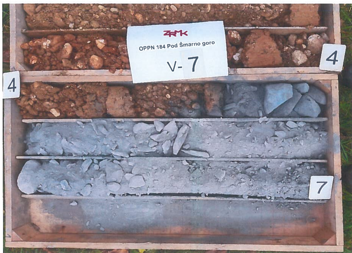
Slika 15: Sondažna vrtina V-7 (4,0 m – 7,0 m)
