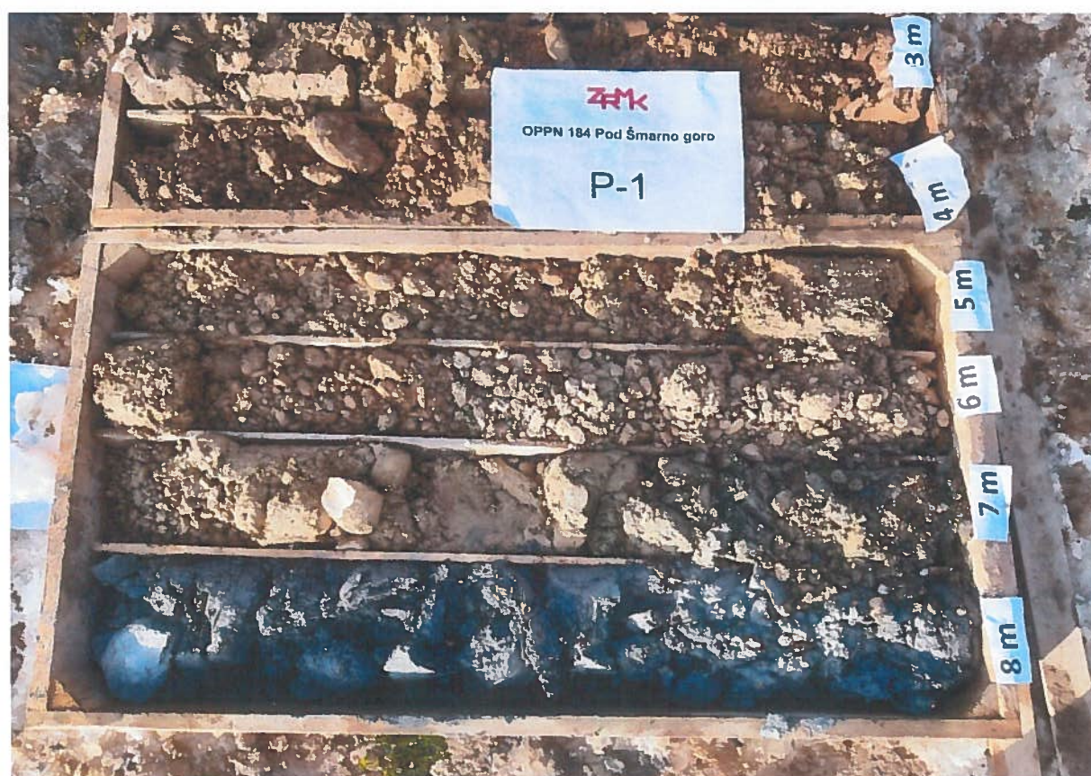
Slika 2: Sondažna vrtina P-1 (4,0 m – 8,0 m)
