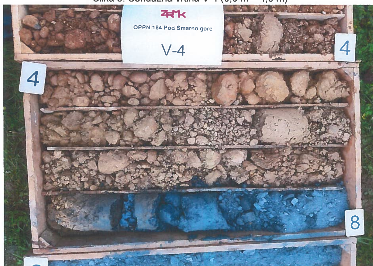
Slika 6: Sondažna vrtina V-4 (4,0 m – 8,0 m)
