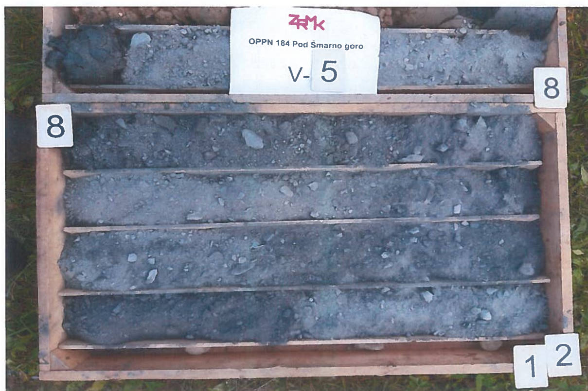
Slika 10: Sondažna vrtna V-5 (8,0 m – 12,0 m)
