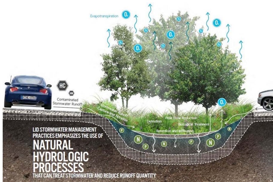
Slika 42: Shema upravljanja s padavinsko vodo z uporabo naravnih hidroloških procesov (Vir: B. Collett, V. Friedmann, W. Miller: Low impact development opportunities for the planet region, Knoxville-Knox County Metropolitan Planning Commission, 2013)
